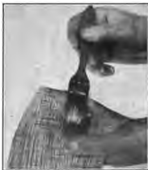
Fig. 70. Placing Shellac on Cloth
